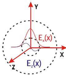
Fig.3 Coordinate system used. X-polarized horizontal field component  $E_x(x)$  is in a loop plane. Field z-component  $E_z(x)$  is anti-symmetrical function of x unlike symmetrical main field distribution.
